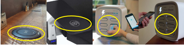
Fig. 5: Illustration of public wireless charging stations and power bank rental services. An attacker can maliciously compromise these facilities to use their coils to capture EM emanations.
